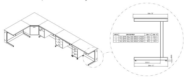
Drainage gradient should be well adjusted throughout the length of table and should have horizontal supports for drainage systems. The structure should have a removable back panel to provide access for maintenance throughout the length of table. The C-frame shall also have skirting at back bottom side. It should be suitable for sitting and standing nominal heights of 750mm & 900mm respectively. The nominal table depths should be 620 mm, 770 mm and 920 mm for wall side and 1240mm,
