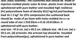
59.5 cm. (d) armrests: the armrest top should be moulded from polyurethane(pu), upholstered in pure leather and mounted on to a drop lift adjustable type tubular armrest support made of 03.81±0.03 cm x 0.2±0.01 cm thk m.s e.r.w tube having chrome plated finish.the armrest height adjustable up to 6.5±0.5cm in 5 steps. active bio-synchro mechanism: the adjustable tiltng mechanism should be
