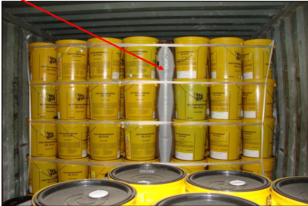
Stack of bucket & Dunnage Air Bag with secured straps while unloading of truck
